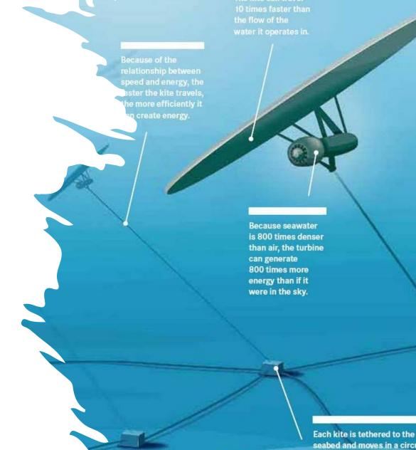
Each kite is tethered to the seabed and moves in a circular pattern, converting tidal currents into energy.
